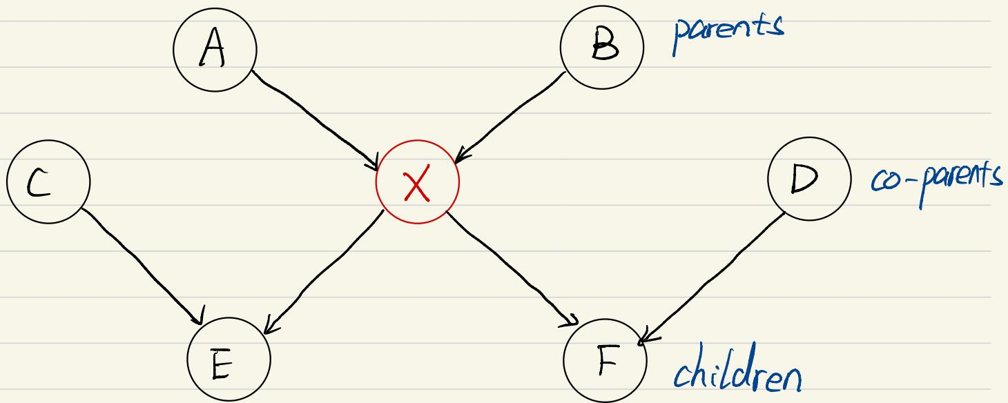
A node conditioned on its Markov blanket is independent from all other nodes in the graph.
