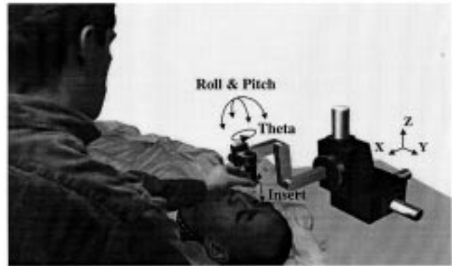
Fig. 2. The steady-hand concept as applied to retinal microsurgery.
