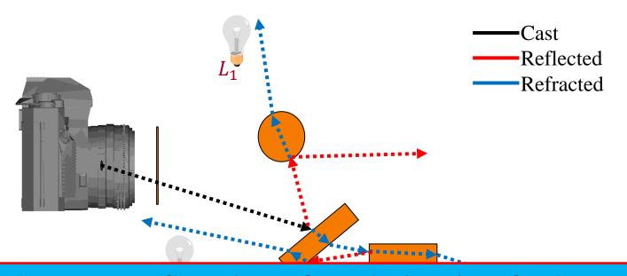
Note that we do not cast reflected rays from the interior of a shape. (i.e. if the dot-product of the normal with the ray direction is positive)
