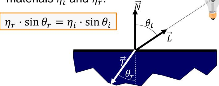
The index of refraction of air is  $\eta = 1$ .
