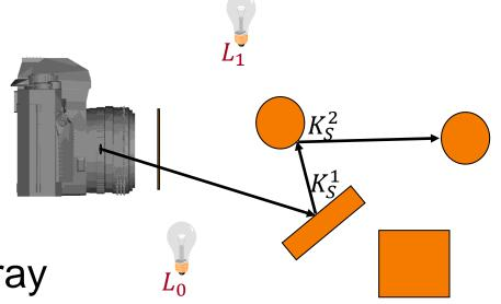
⇒ The second reflected ray should be cast if it can reflect at least  $\frac{\text{cut-off}}{\kappa^{\frac{1}{2}}}$  of the local intensity
