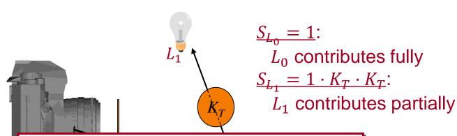
For solid models we can use the distance, d, travelled through the surface instead:  $S = e^{-d \cdot K_T}$
