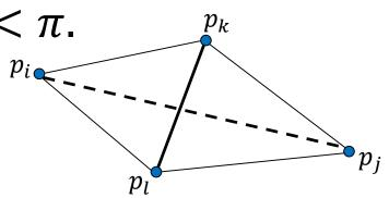
We can perform an *edge-flip* to change a non-locally Delaunay edge into a locally Delaunay edge.
