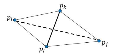
We can perform an *edge-flip* to change a non-locally Delaunay edge into a locally Delaunay edge.
