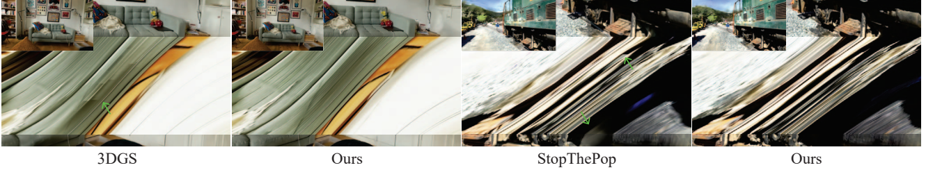
Figure 7. Here we show epipolar plane images [6] to visualize popping in 3DGS [23] and StopThePop [36]. We recorded sequences of images while rotating the camera in the berlin [4] (left) and train [26] (right) scenes. The region in the middle are the epipolar plane images, with green arrows highlighting discontinuities in the color caused by popping/blend order artifacts. Our method lacks these horizontal discontinuities. Contrast and brightness have been boosted here for visibility’s sake. See the supplemental video for more.
