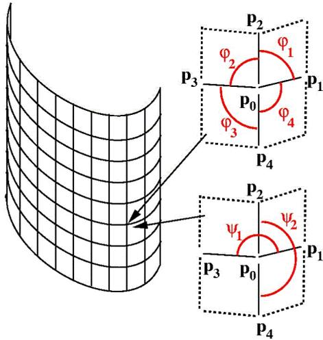
**Figure 4:** Shear and bend energy in a particle system (image by Eberhardt [14])
