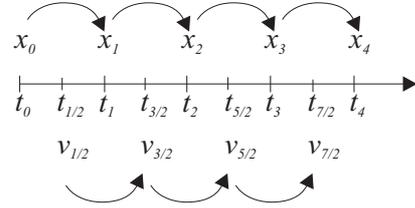
Figure 12: Staggered grids for the Verlet method.
