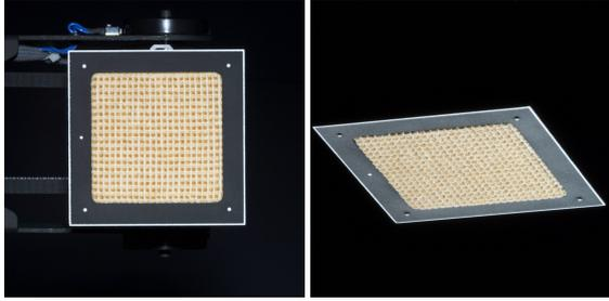
**Figure 5:** Sample holder with the PROPOSTE sample. The left image shows the frontal view ( $\theta = 0^\circ$ ,  $\phi = 0^\circ$ ); the right image shows ( $\theta = 60^\circ$ ,  $\phi = 342^\circ$ ). White point and border markers are clearly visible.
