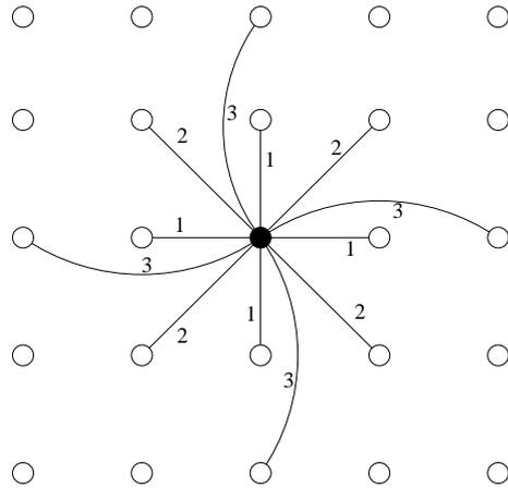
**Figure 2:** Provat's mass-spring system with (1) structural springs, (2) shear springs, and (3) bending springs
