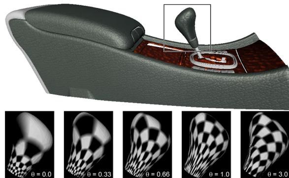
**Figure 9:** Top: BTF textured gear box model (courtesy of DaimlerChrysler) based on the computed parameterization. Bottom: the effect of varying  $\theta$  is shown: for  $\theta = 0$  a conformal mapping results, for  $\theta = 1$  angle and area preservation are equally important. With growing  $\theta$  area preservation improves.
