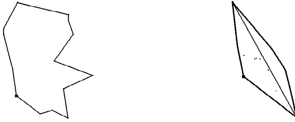
Fig. 7. Starting in (a) with a border subproblem, we look for a new Delaunay edge of a point q by using inversion around q to move to the dual problem of finding convex-hull edges. This is shown using thick lines in (b). The new Delaunay edge we pick is to the point farthest from the line between the points preceding and following q , shown in a thin line.
