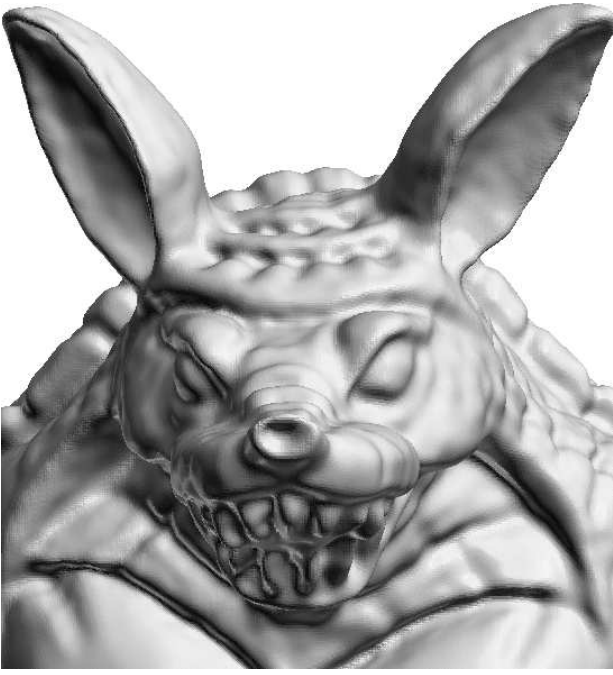
Fig. 8. Adaptive PU + RBF reconstruction of the Armadillo part used also in Fig. 6.
