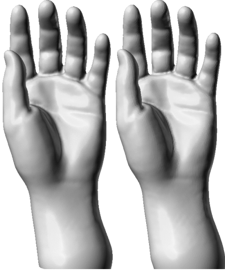
Fig. 11. To compare our method with FastRBF [9] we use the Hand model (13,348 points). Left: the surface is approximating by FastRBF (computational time is 30 sec., 26,696 RBFs are used to represent the model). Right: the surface is interpolated by our method (computational time is 7 sec., the model is represented by the sum of 18,647 basis functions).
