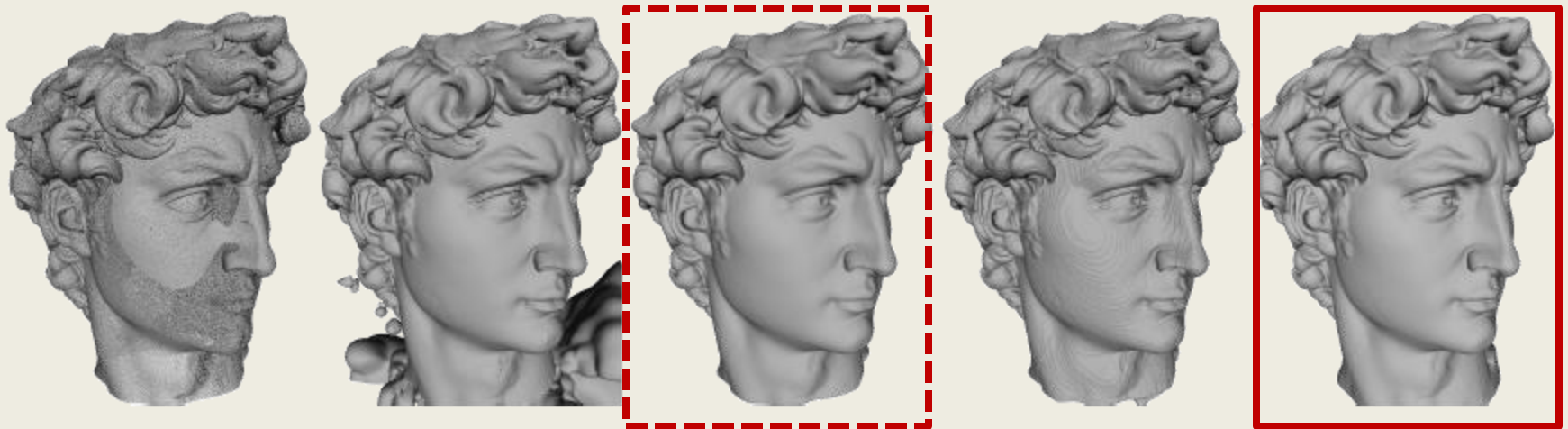
Figure 5: Input point cloud (leftmost) of David's head, and reconstructions using (from second-left to right) MPU, Poisson, D4 Wavelets, and our SSD reconstruction.
