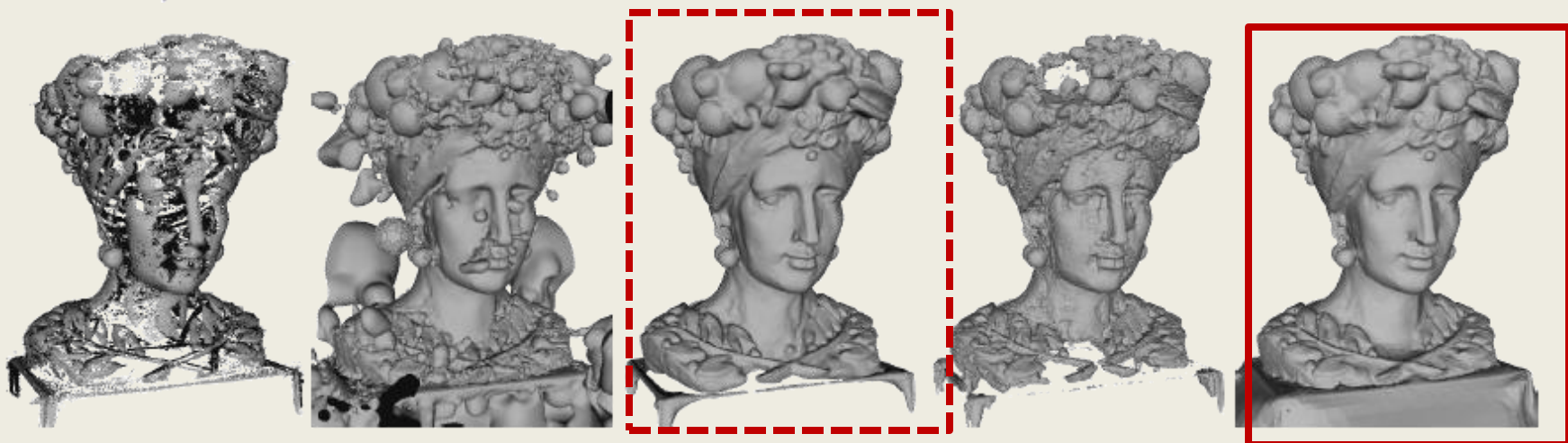
Figure 8: Input point cloud (leftmost) of the Chiquita model, and reconstructions using (from second-left to right) MPU, Poisson, D4 Wavelets, and our SSD reconstruction.
