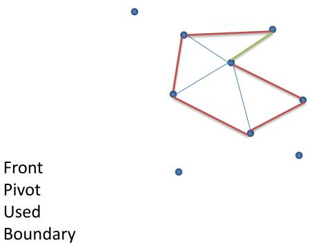
The algorithm takes in a set of oriented points and produces a mesh in linear time.
