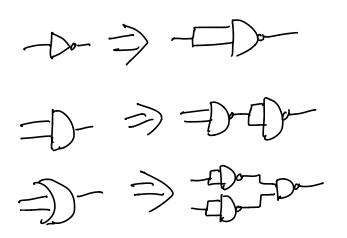
So given circuit **C**, first transform it into NAND-only circuit.
