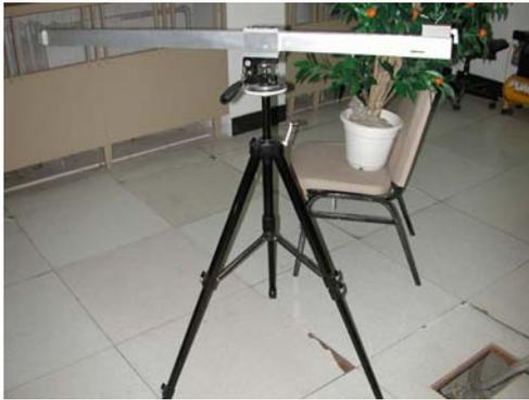
Fig 8. Our 1D camera self-calibration system: with a straight bar mounted on a tripod.
