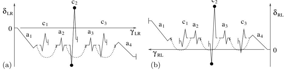
**Fig. 3.** Monitoring the delay on all acyclic paths of  $A_1^{(n)}$ , exploring (a) forward from initial states and (b) backward from final states. In (b), the sign of the delay is negated. Global extrema are marked. Gaps denote points where the search algorithm backtracked to avoid completing a cycle. Dashed arrows lead from a choice point to alternative paths that are explored after backtracking.
