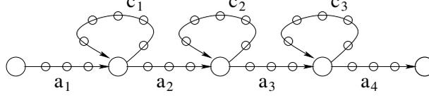
**Fig. 1.** An example  $n$ -WFSM  $A_1^{(n)}$ , having four acyclic factors  $a_h$  and three cycles  $c_h$  with positive delay.
