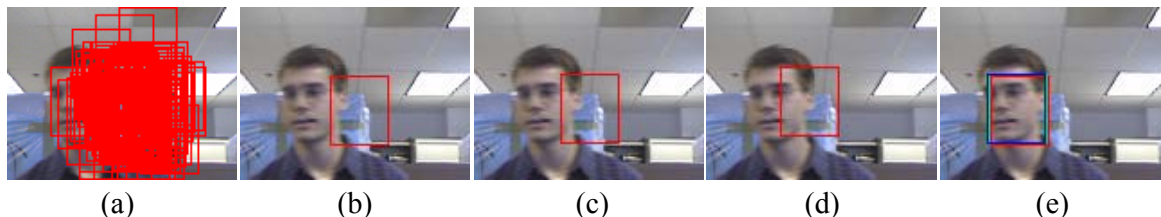
Fig. 3. An example of tracking a face with a weak dynamic model: (a) 100 particles configurations out of the 5000 particles. (b) to (d) The results using the color histogram based similarity measure with (b) 4x4x4 bins; (c) 8x8x8 bins; and (d) 16x16x16 bins. (e) The results for the proposed method with k=5 , k=7 and k=9 .
