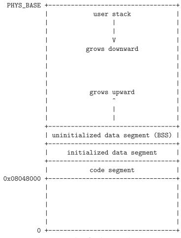
In this project, the user stack is fixed in size, but in project 3 it will be allowed to grow. Traditionally, the size of the uninitialized data segment can be adjusted with a system call, but you will not have to implement this.
