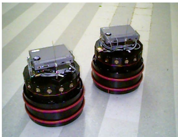
Figure 2: Two Nomad 150 robots programmed to forage using TeamBots.
