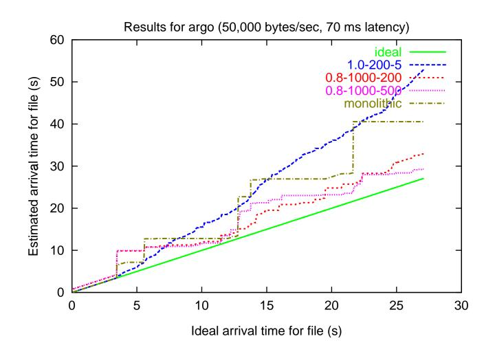
Expected file arrival times vs. ideal for drawtest: 50,000 bytes/second bandwidth, 70 milliseconds latency
