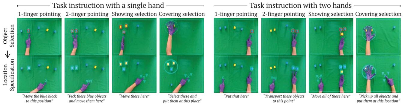
Fig. 2. Our interaction convention for multimodal instruction of pick-and-place tasks. It supports the use of indicative gestures with one or two hands for object selection and for location specification, as well as the use of verbal commands to describe task actions and object features.
