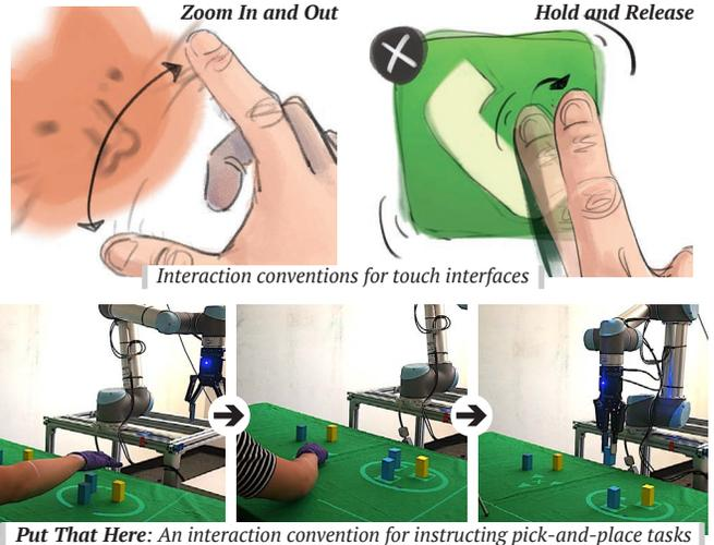
Fig. 1. Similar to how *interaction conventions* can be used to structure human-computer interactions (Top), we contend that appropriate interaction conventions can enable productive human-robot interactions. We present a real-time, interactive system that implements an interaction convention through which users use multimodal behaviors to instruct a robot manipulator in performing pick-and-place tasks (Bottom).
