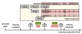
Figure 6: Periodic heap snapshot collection.
