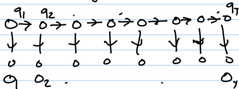
Forward variable  $\alpha_t(i)$  is prob. of observing the partial sequence  $(O_1, \dots, O_t)$  and being in state  $S_i$  at time  $t$ , (given the model  $A$ )
