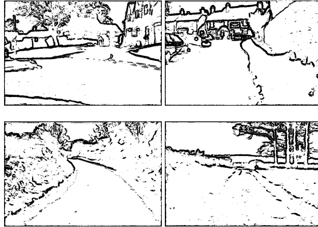
Figure 7: The edges obtained by our \log P_{on}/P_{off} criterion for the Sowerby images shown earlier. The edge filters used the modulus of the Gaussian with full colour and combining scales \sigma = 1 and \sigma = 2 .
