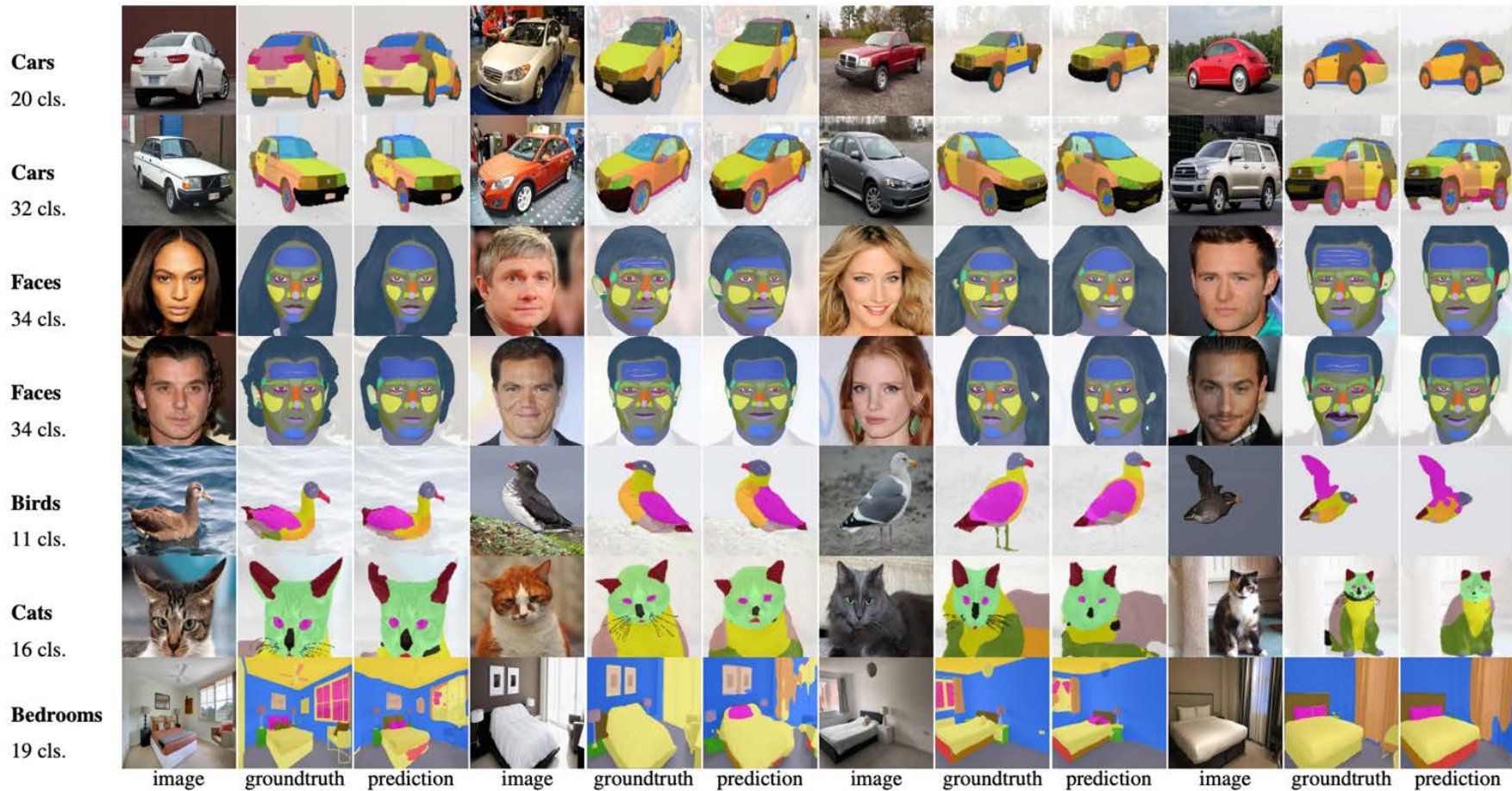
Figure 7: Qualitative Results: We visualize predictions of DeepLab trained on DATASETGAN’s datasets, compared to ground-truth annotations. Typical failure cases include parts that do not have clear visual boundaries (neck of the cat), or thin structures (facial wrinkles, bird legs, cat whiskers).
