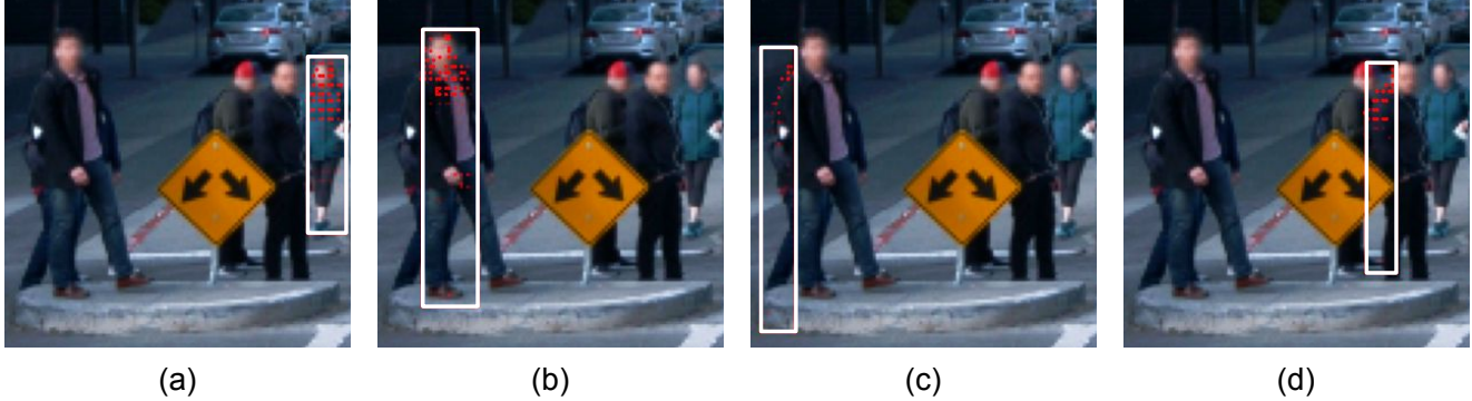
Figure 5. The attention map visualization for LearnableAlign. For each subfigure, we study one 3D point pillar, which is marked by the white box in the 2D image. The important region indicated by the attention map is marked by red points. We have two interesting observations: first, as shown in (a) and (b), LearnableAlign usually attends to the heads of the pedestrians, probably because the head is a discriminative part of a human from camera image (it is difficult to recognize a head according to lidar signals); second, as shown in (c) and (d), LearnableAlign also attends to object extremities (such as the back), which strives to use the high-resolution camera information for predicting the object boundary to get accurate object size.
