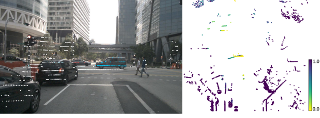
Figure 3. Illustration of the probabilistic motion masking. Left: the projected points with color encoding optical flow (ego-motion factorized out) on the front image. Right: part of the point cloud and the probabilities of nonempty pillars being static.
