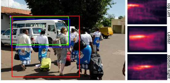
Figure 3: Example of robust bounding box voting results. Blue box: ground truth; red box: bounding box by Faster R-CNN; green box: bounding box generated by robustly combining voting results. Our proposed part-based voting mechanism generates probability maps (right) for the object center (cyan point), the top left corner (purple point) and the bottom right corner (yellow point) of the bounding box.
