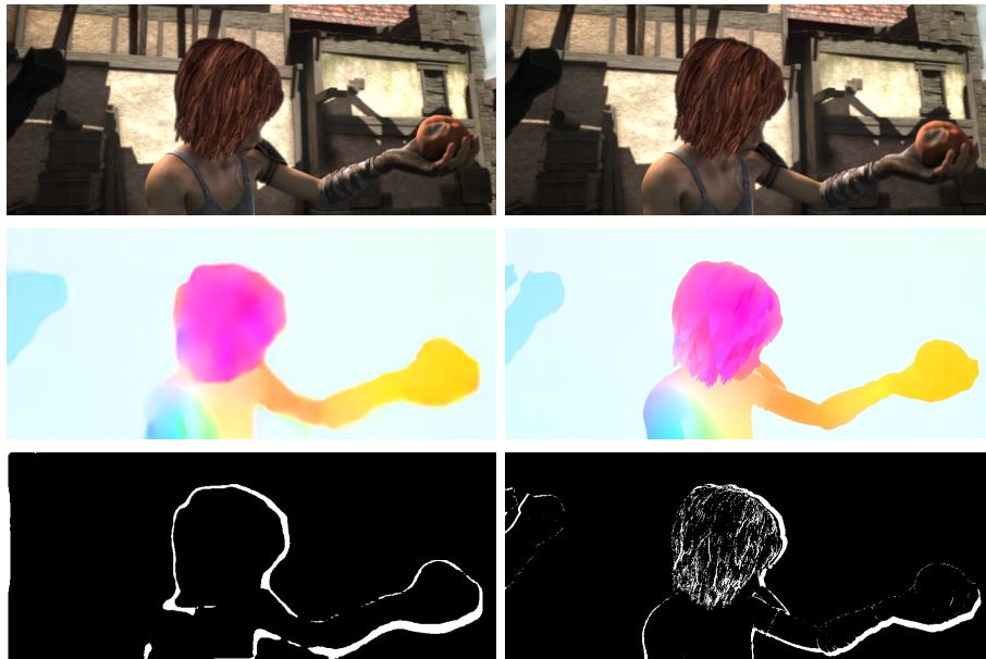
Figure 6: Qualitative results of our full model method on the MPI-Sintel dataset. From the second row to the third row, the left images are the estimated optical flow and occlusion mask respectively. The right images are the corresponding ground truth. The mask is demonstrated by the threshold 0.5.
