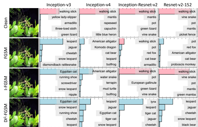
Figure 1. The comparison of success rates using three different attacks. The ground-truth “walking stick” is marked as pink in the top-5 confidence distribution plots. The adversarial examples are crafted on Inception-v3 with the maximum perturbation \epsilon = 15 . From the first row to the third row, we plot the top-5 confidence distributions of clean images, FGSM and I-FGSM, respectively. The fourth row shows the result of the proposed Diverse Inputs Iterative Fast Gradient Sign Method (DI 2 -FGSM), which attacks the white-box model and all black-box models successfully.
