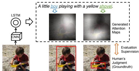
Figure 1: Image captioning models (Xu et al. 2015) can attend to different areas of the image when generating the words. However, these generated attention maps may not correspond to the region that the words or phrases describe in the image (e.g. “shovel”). We evaluate such phenomenon quantitatively by defining attention correctness, and alleviate this inconsistency by introducing explicit supervision. In addition, we show positive correlation between attention correctness and caption quality.
