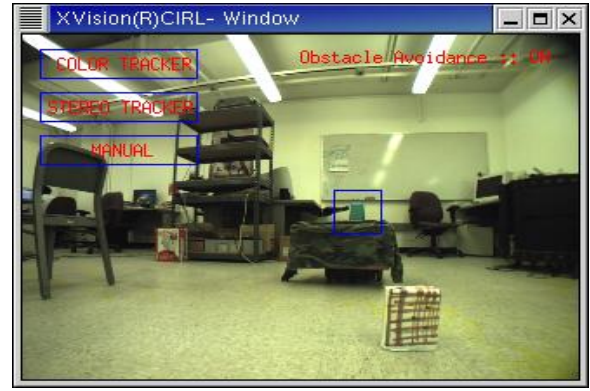
Figure 5: User-interface while robot is navigating towards the tracked object
