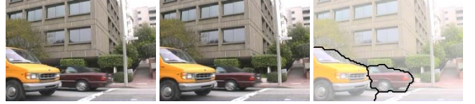
Figure 10. Motion segmentation with static camera and two moving cars. I_1 (left), I_2 (middle), segmentation (right).
