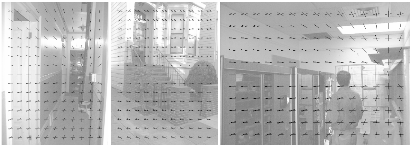
Figure 8: Another indoor (left panel) scene, its exterior (right panel), and another indoor scene (right panel). Same conventions as above. The vanishing points are estimated to within 5^\circ (perfectly adequate for our purposes). Note poor quality of the indoor image (i.e. over-exposed). (Indoor 23,8 and Outdoor 12).
