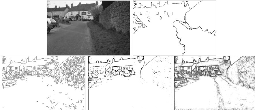
Figure 1: A typical Sowerby image (top left panel) with its ground truth segmentation (top right panel) and its segmentation using the Canny edge detector (bottom left panel) and by statistical edge detection (bottom centre panel). Statistical edge detection has fewer false negatives in the textured regions and is also better at detecting edges which are partially defined by texture. By contrast, the Canny detector is slightly better at precision of certain edges. The log-likelihood ratios are also shown (bottom right panel).
