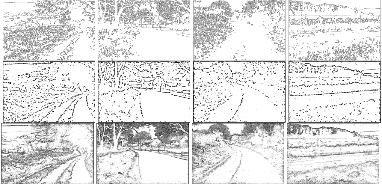
Figure 17: Top panels shows edges detected using the Canny edge detector. The centre panels shows the output of statistical edge detection on the same images. The bottom panels show the log likelihood ratios which give a measure of edge strength. See figure (7) for the images and the ground truth.
