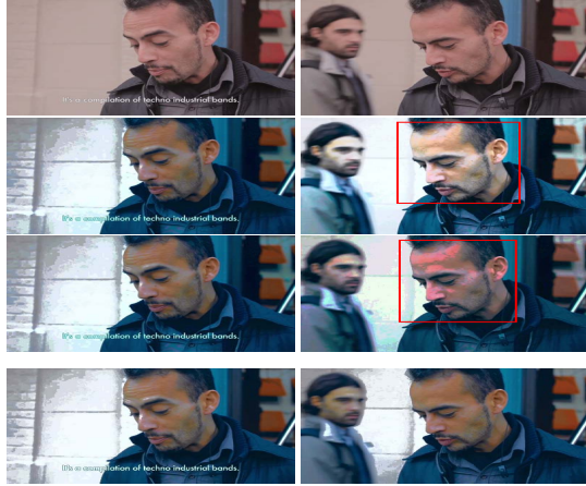
(a) Two example frames from a video. Top to bottom: original input frames, original enhancement results, enhancement results of the algorithm in [6] with multiple key frames, and our results. First column: a non-flickering frame of the video. Second column: a flickering frame of the video. The region in the red box shows unwanted enhancement.
