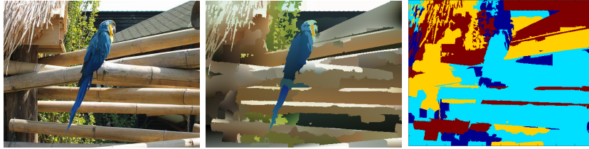
Figure 6: Different segments can have different polynomial order k . Left: original. Center: polynomial base approximation. Right: order of the polynomial, where: dark-blue: k = 0 , light-blue: k = 1 , yellow: k = 2 ; red: k = 3 .
