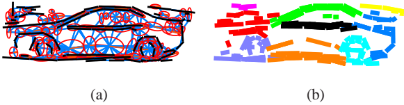
Fig. 13: Pairwise clustering is used to discover object parts: first the object contours are broken into straight segments, which are seen as nodes on a graph. Ridges are shown as ellipses whose width is proportional to the scale of the ridge. Nodes are connected with edges based on continuity and parallelism. The affinity among nodes is estimated using statistical and geometric information. The object parts shown on the left are obtained using Affinity Propagation.
