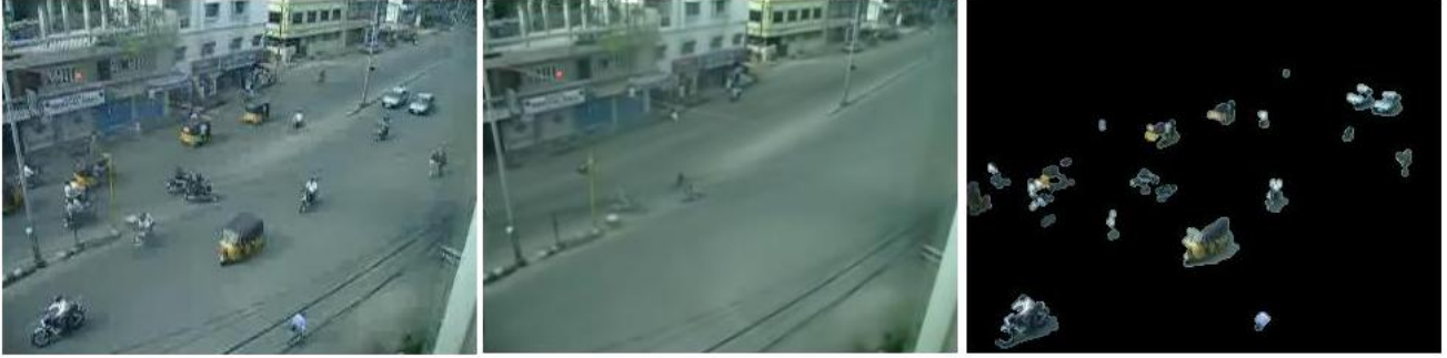
Figure 3. Above we show (From left to right) a rectified image, followed by our learned background and finally show our segmented image.
