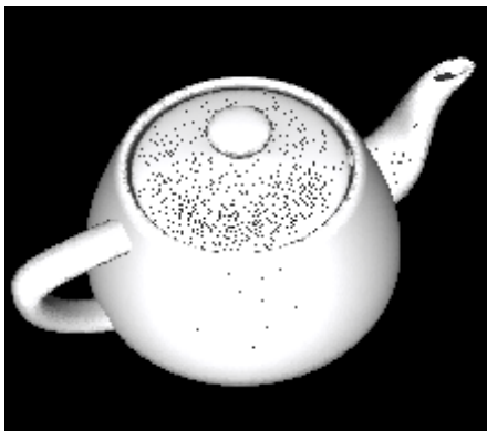
Figure 9: Holes on the Teapot model when the points are rendered with a point size just one less than the computed one
