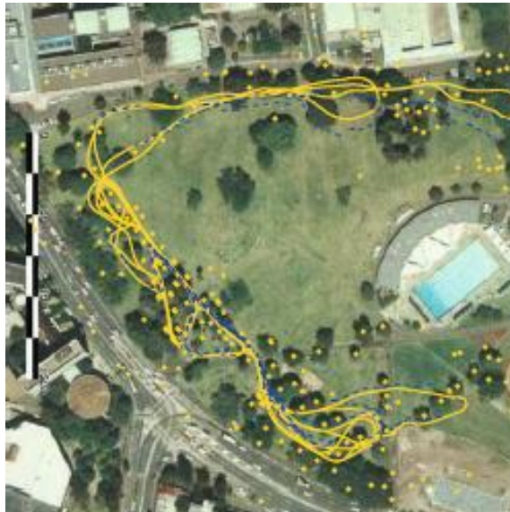
(a) Vehicle path predicted by the odometry
