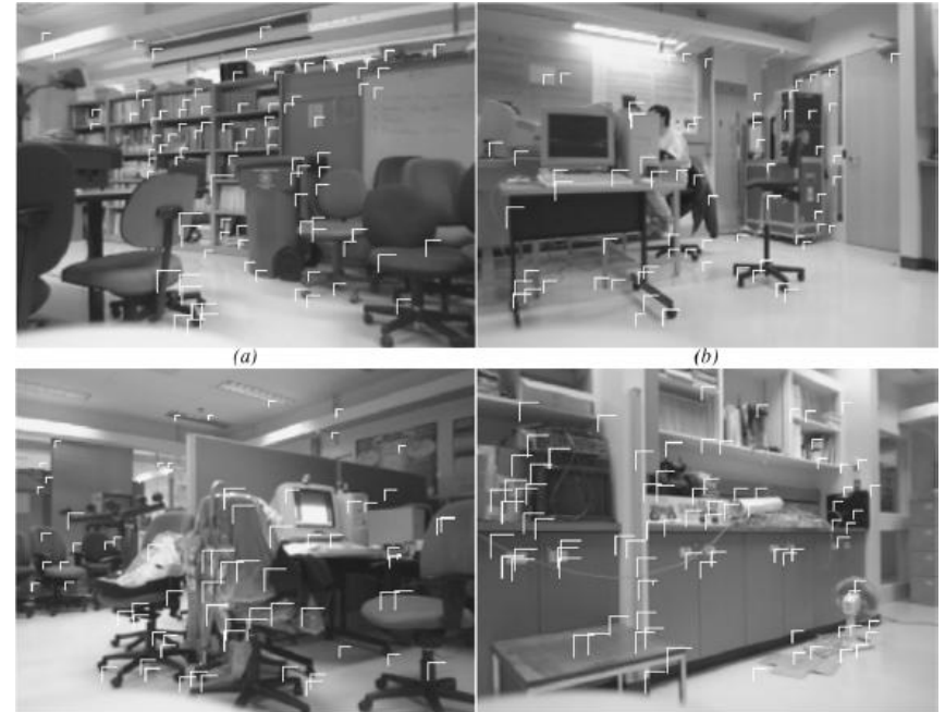
SIFT landmarks from stereo camera Disparities are indicated by lines
