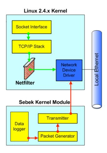
Conceptual representation of Sebek packet generation. Note how packets created by Sebek bypass the stack and go directly to the network device driver. This makes it far more difficult for attacker to detect Sebek activity.
