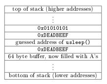
Figure 2: Stack after one probe
