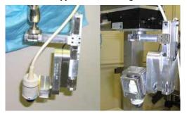
**Figure 2:** TRCM with US Probe on Passive Arm (left) and on a 3DOF cartesian base robot(right)
