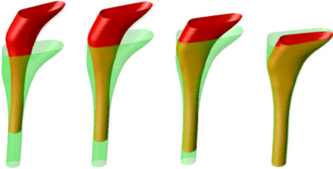
Figure 2: Example of an insertion sequence of an implant stem (dark body) tightly fit into a canal (translucid body) from the initial inserted configuration (left) to the final free (right) configuration.
