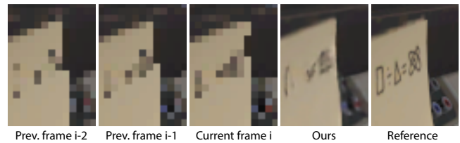
Fig. 12. Failure case. When the multi-frame inputs do not contain enough information of the underlying scene, i.e., the text on the sticky note, the method fails to recover the full details of the text.
