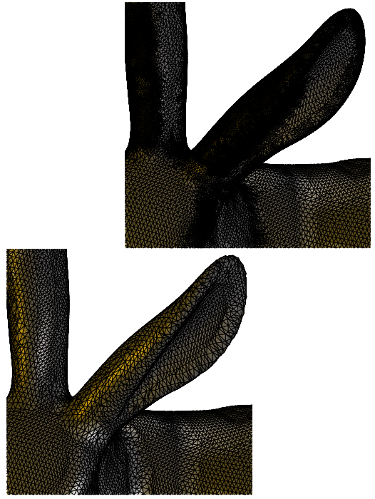
Figure 5: The resulting surface mesh (top) from an adaptive algorithm is compared with the corresponding grid of an evolution with fixed triangulation (bottom). The areas of high curvature are clearly visible as refinement regions.
