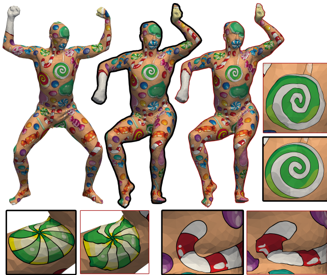
Figure 8: Comparison of our map (bold) to the ground-truth map of SCAPE [Angelov et al. 2005] (red frame). Left: textured source mesh. Note that the maps are similar but SCAPE’s mapping lacks smoothness and exhibits high distortion.
