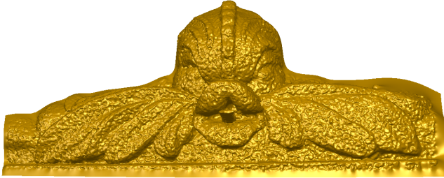
Figure 6: An ‘exact’ fit, to an accuracy of 10^{-6} mm, of an RBF to the noisy LIDAR data studied in Figure 7.
