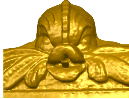
Figure 11: Smoothing using a discrete approximation to the multiquadric smoothing kernel.
