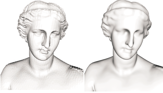
Figure 4: The effect of different values for parameter h . A point set representing an Aphrodite statue defines an MLS surface. The left side shows an MLS surface resulting from a small value and reveals a surface structure resulting from the wood carving. The right side shows a larger value for h , smoothing out small features or noise.
