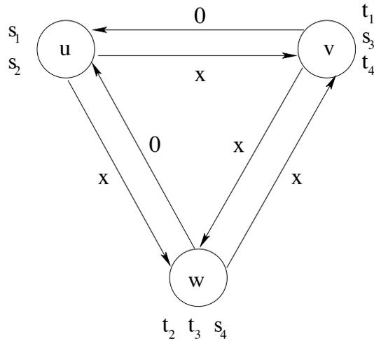
In this example every demand has a one-hop path using an edge with cost function  $x$ , but they also have 2-hop paths. First, note that if every player uses their single-hop path then each player pays 1, so the cost of this flow is 4 (this is in fact the optimum flow, although we don't need to prove that).
