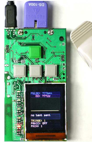
Figure 4: Custom vital sign collecting hardware developed for MEDiSN.
